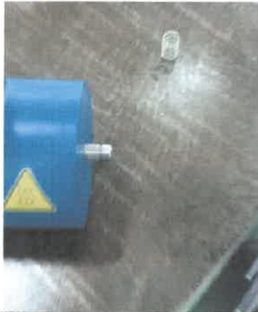
步骤 1: 用一字螺丝刀拆掉卡簧和弹簧
